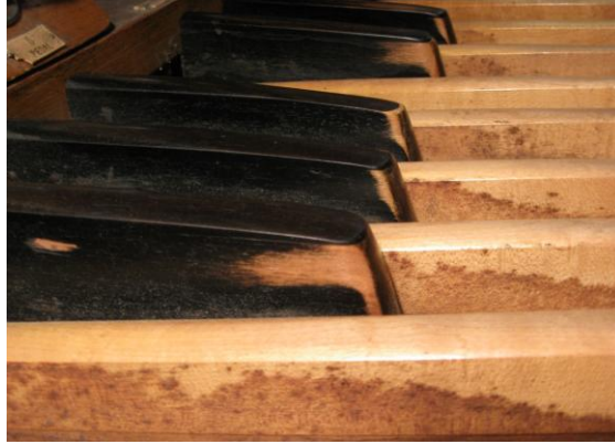
Figure 9: The pedal keys showing wear as well as stains from mold and mildew.
