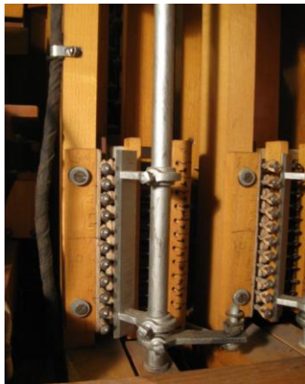
Figures 12 and 13: Parts of the Combination Action, and two large solenoids which operate part of it.
