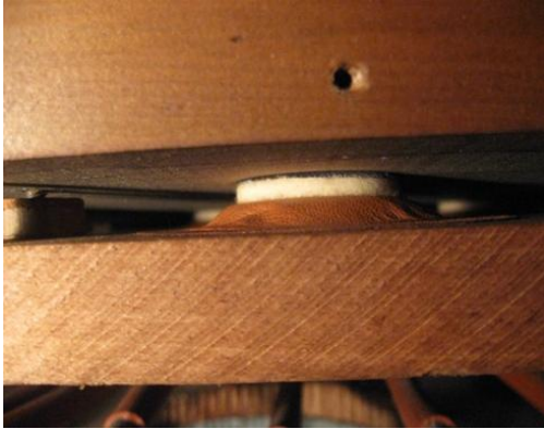
Figure 44: Pedal offset chest with releathered pouch.
