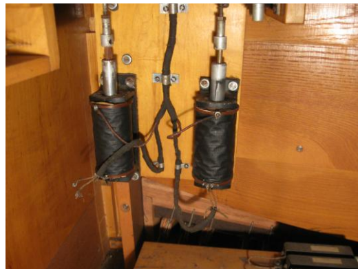
Figures 12 and 13: Parts of the Combination Action, and two large solenoids which operate part of it.
