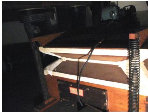
Figure 6: When the wind regulator is filled with pressurized air, the head rises, expanding the ribs.
