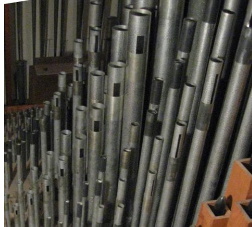
Figure 38: Metal pipes with coke tin tuning slides. Wooden pipes with stoppers lower right.
