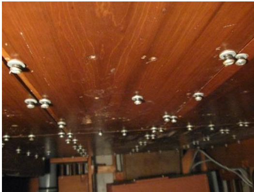
Figure 41: Underneath the Swell chest showing the bottom boards.
