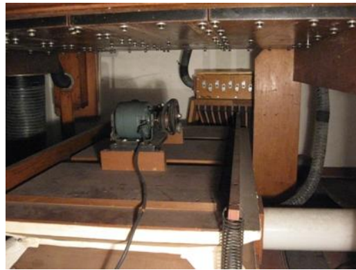
Figure 36: The tremulant motor on the Great wind regulator.
