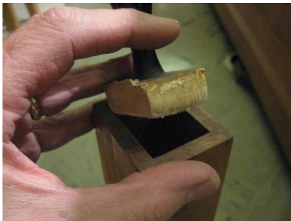
Figure 40: Stopper of a Stopped Diapason pipe showing old, dried leather.
