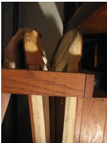
Figure 34 and 35: Concussion bellows for the Swell and Great windchests.
