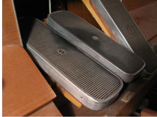
Figure 11: The pedals for the Great and Swell expression shades; the crescendo pedal.
