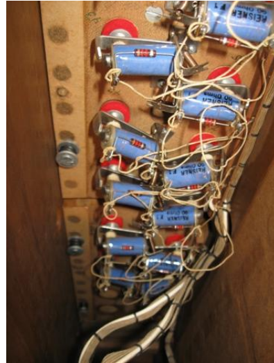
Figure 42: With a bottom board removed, a view of the Swell chest, showing the direct valve action.
